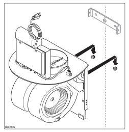
Place the upper holes of the motor assembly over the 2 mounting screws in the wall.
